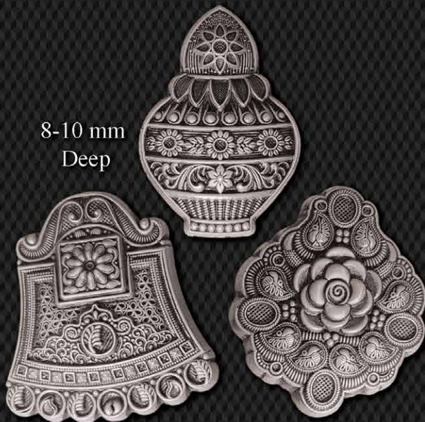
Stamped on Compound Die 0.31 mm (30 Gauge) Silver sheet (Weight reduced by 30%)
